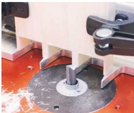
▲ It makes a finer pin profile on through dovetails
